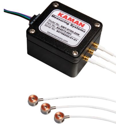
In many applications the actual motion to be monitored can be very small. A full scale calibration of 100 microns is not unusual, and with a full scale output of 10VDC, sensitivity is high, in this case 100mV/micron.
