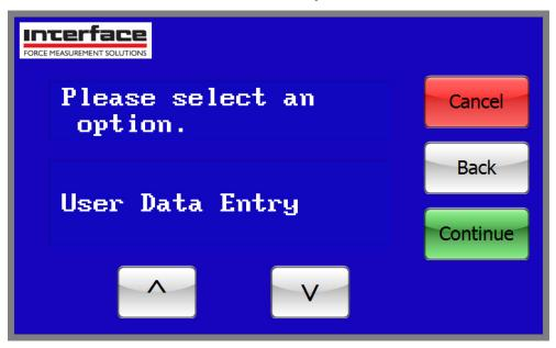
For this menu and its sub-menus, the down button navigates forward through the list, and the up button navigates backwards.
