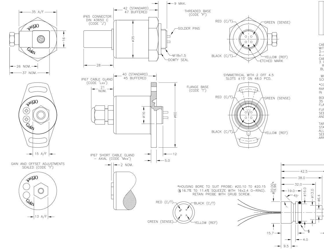
CONNECTIONS BETWEEN PROBE AND ELECTRONICS MODULE: FOUR WIRES; RED, BLACK, GREEN AND YELLOW, LENGTH: 300, CROSS SECTION: 0.25mm<sup>2</sup>, WIRES POTTED IN PROBE HOUSING. INTERCONNECTIONS MUST BE PROTECTED FROM WATER INGRESS AND STRAIN RELIVED.
